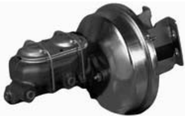
Master cylinder with vacuum booster assembly which supplies power assist to brakes.
