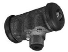
Carefully, remove wheel cylinder.
